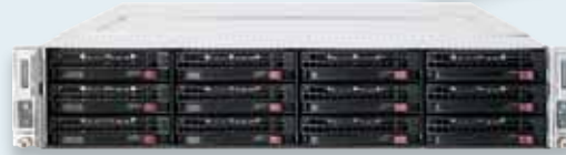
12x 3.5" hot-swap SATA hard drives support (6x per node)
